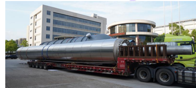
Picture of Guanxi Henyi ammonia converter basket manufactured by Anchun
